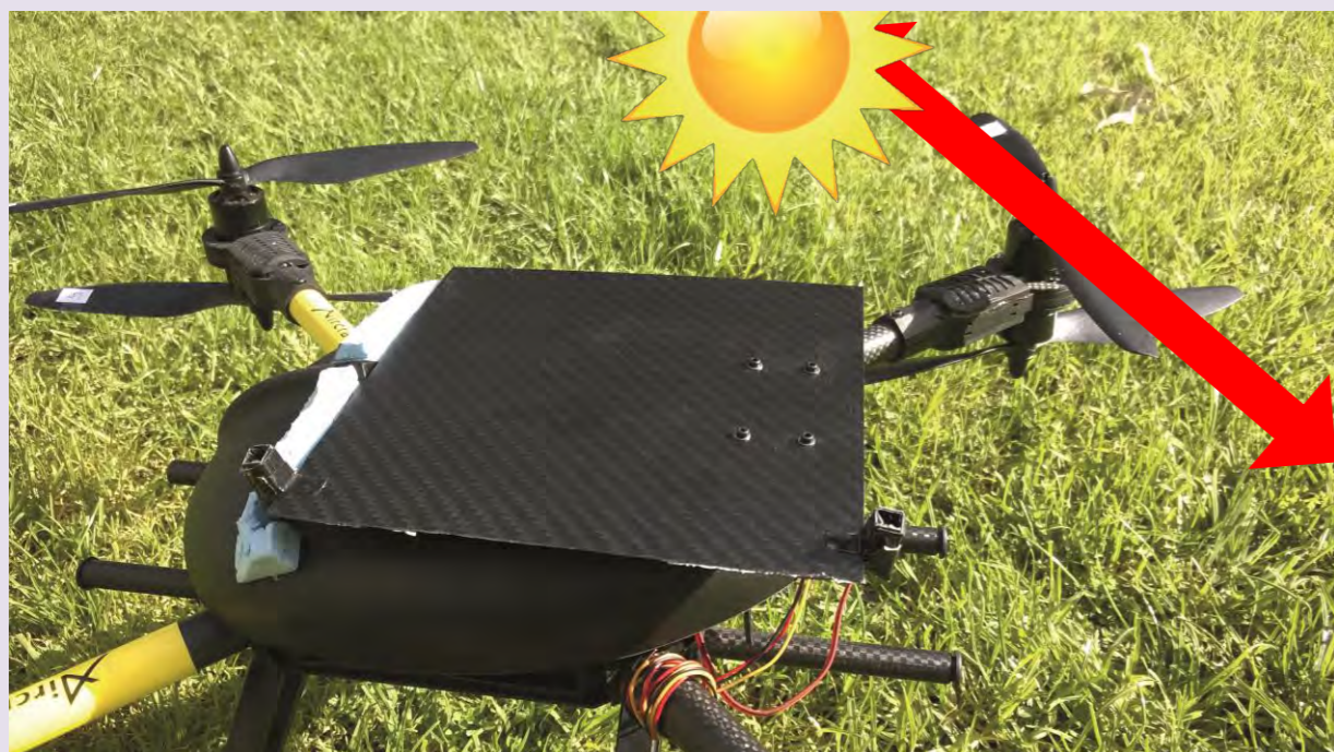
The main panel uses light sensors to track the sun's movement in the sky in the vertical plane during charging to maximize energy harvesting.
