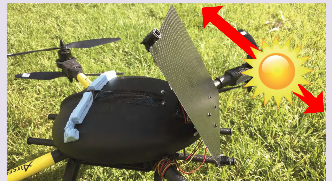
The main panel uses light sensors to track the sun's movement in the sky in the vertical plane during charging to maximize energy harvesting.
