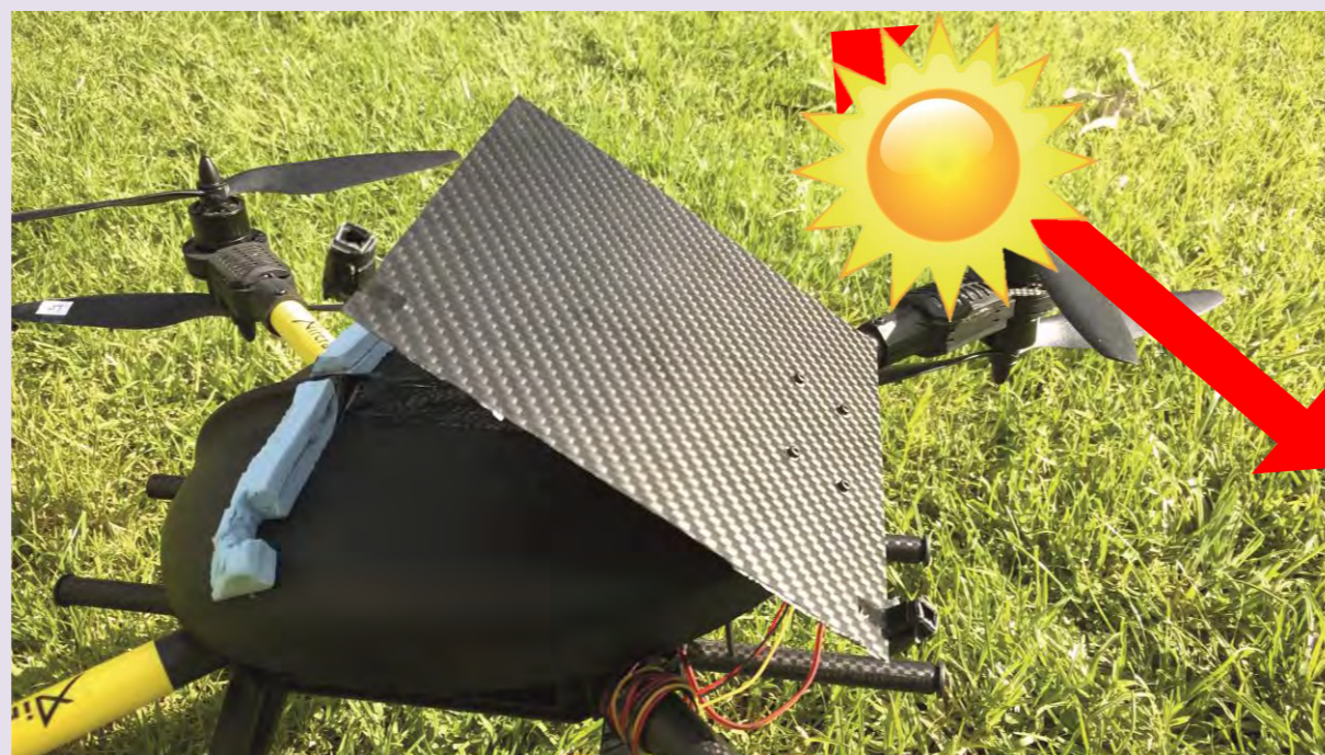
The main panel uses light sensors to track the sun's movement in the sky in the vertical plane during charging to maximize energy harvesting.
